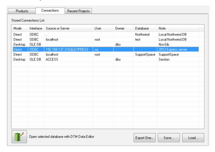
If you have installed DTM Data Editor the program allows you to open it for the selected connection.
